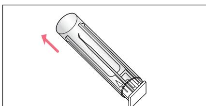
3. Remove the protection tube from the capillary safe.
