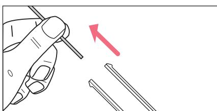
4. Hold the capillary in the middle and pull it out of the capillary safe.
